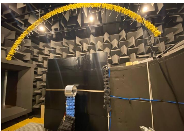
Fig. 1 Experimental setup of a BLI ducted fan in the aeroacoustics wind tunnel at the University of Bristol
